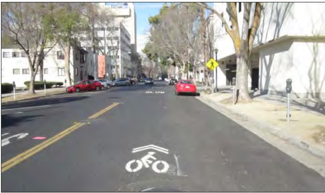
Shared lane markings (Sharrows) indicate a shared lane for cyclists and vehicles and recommended cyclist positioning within the roadway.
