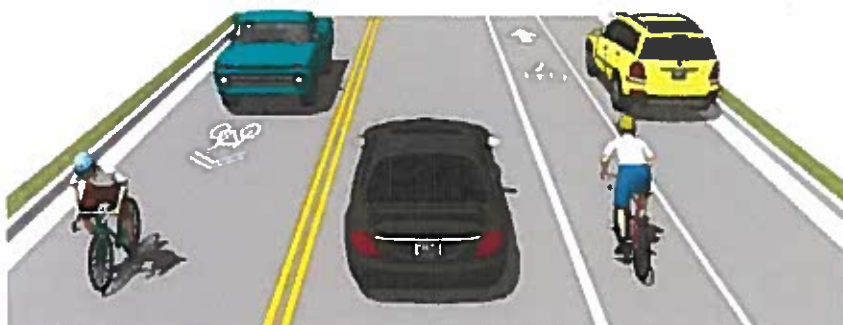
"Climbing lane" configuration: Class 2 lane uphill and Class 3 route downhill with "Sharrows" positioned at least four feet from curb (per California MUTCD)
