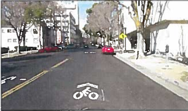
Shared lane markings (Sharrows) indicate a shared lane for cyclists and vehicles and recommended cyclist positioning within the roadway.
