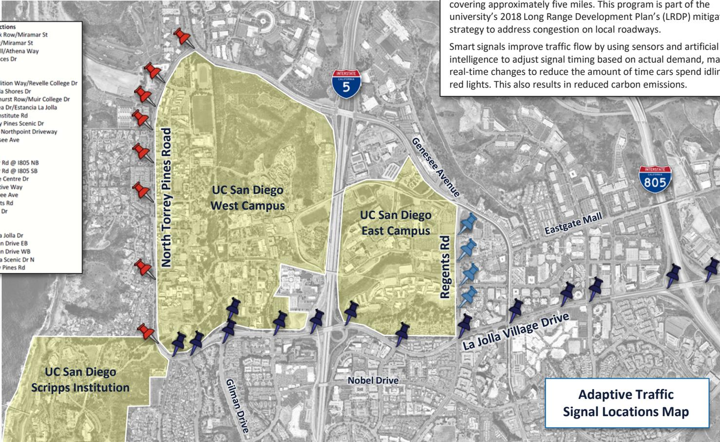
UC San Diego will implement adaptive traffic signal controls (“smart signals”) at 26 intersections along roadways surrounding campus, covering approximately five miles. This program is part of the university’s 2018 Long Range Development Plan’s (LRDP) mitigation strategy to address congestion on local roadways.
