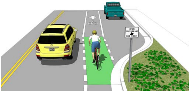
Colored bicycle lane at location with high potential for conflict with motor vehicles
