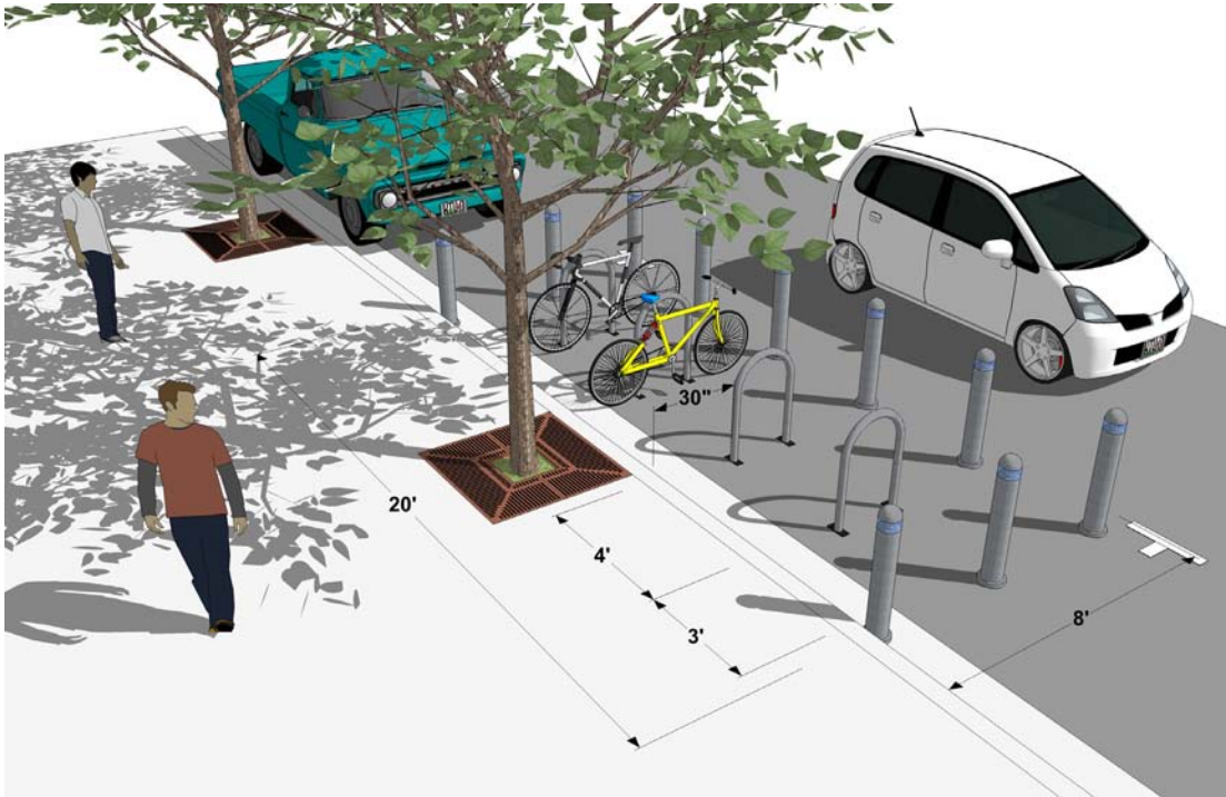
Bike corral dimensions - Converts one car parking space into 8-10 bike spaces
