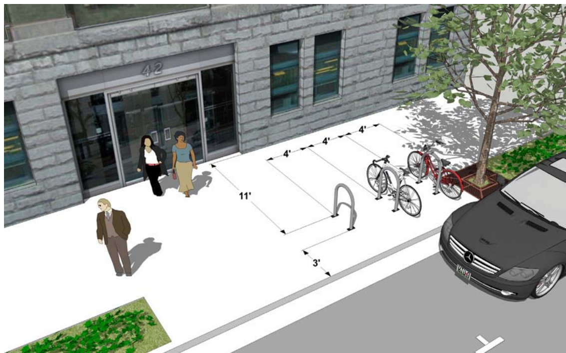
Bicycle rack dimensions for installations perpendicular to curb
